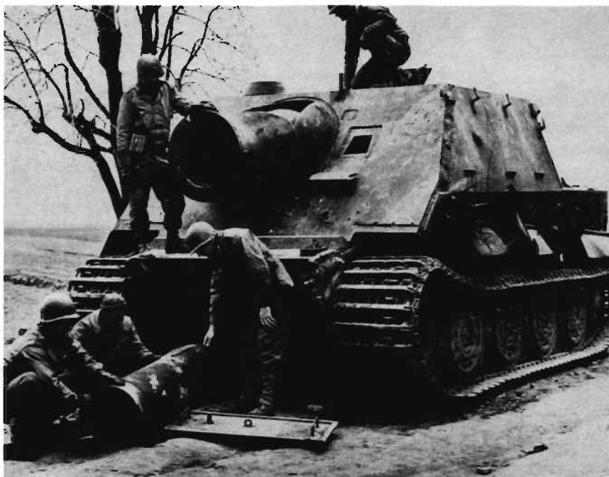
U.S. soldiers examine an unusual German vehicle, the 305-mm assault mortar mounted on a heavily armored Tiger chassis.
