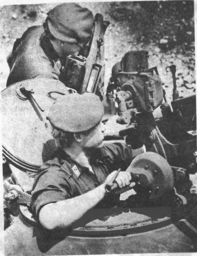
OP-4 people check out the free action on the turret mounted machine gun of the T-62 tank.
